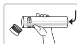
Fig.6 A new ECOCART can be inserted from the opposite end of the holder.
